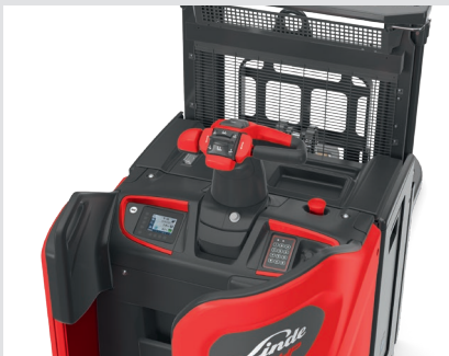
Ergonomic, height-adjustable tiller
