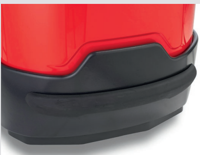
Front cast steel bumper
